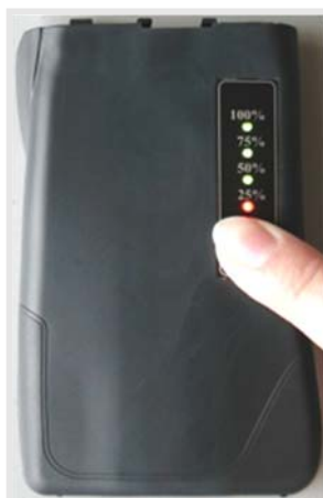
Test of battery charging condition
